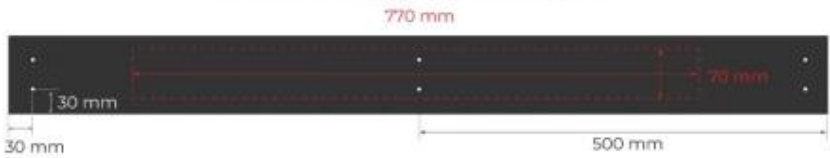
Top view with fixing points and burner cutout with lip in bottom plate
